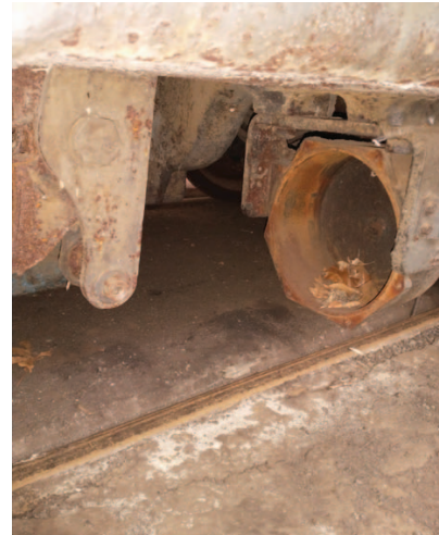
Missing brake cylinder
